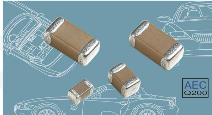
The soft termination MLCC is designed by inserting a conductive silver polymer layer into the typical termination structure. This layer acts as a “cushion” to relieve the stress when the MLCC is in a severe environment. Compared with the other automotive grade AC series, which guarantees a 2mm test board flexure, the AS series can resist at least 5mm for case sizes equals to or smaller than 1210.
